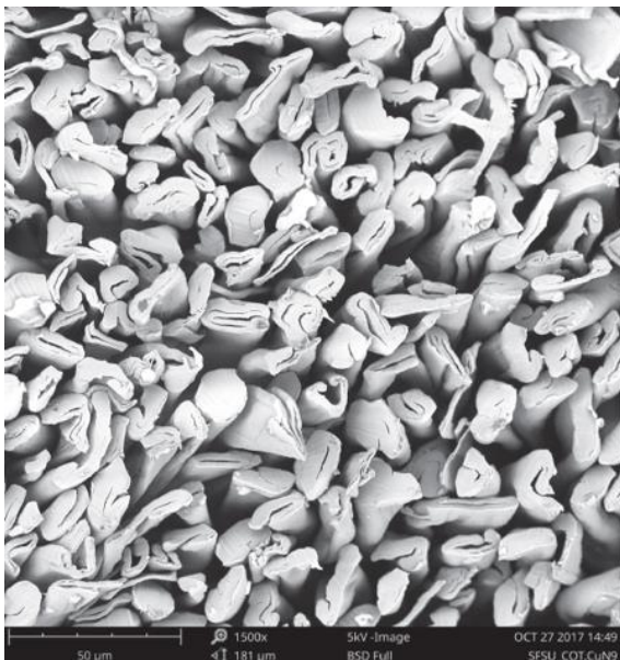
Figures 25 & 26. Cross-section of cotton fibres with a variety of wall thickness showing mature fibres with thick cell wall and a small lumen and immature fibres U shape cross-section with a thin cell wall (1500x) (Markova 2019: 4) with depiction of physical structure of cotton fibres (Markova 2019: 3).
