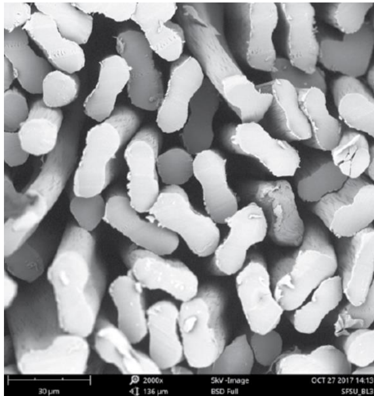
Figure 15. Dog bone cross-section acrylic blanket fibres x2000 MAG. (Markova, I., 2019. Textile Fiber Microscopy: a Practical Approach . New Jersey: John Wiley and Sons, p.132.)
